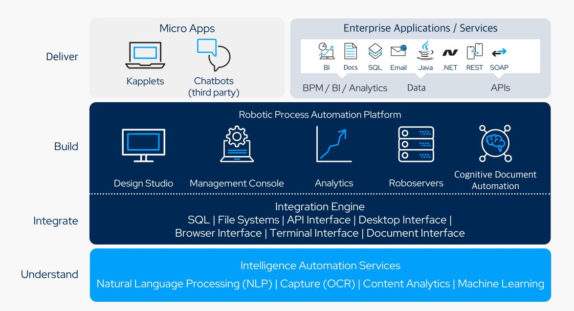
An extensible and versatile architecture for designing, deploying and managing robots. Comes with embedded Cognitive Document Automation capabilities and integrates with business process management and other third-party technologies.
